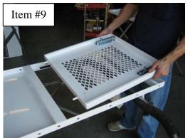
Remove 3<sup>rd</sup> Compartment Bulkhead Emergency Exit Hatch to ease installation.
